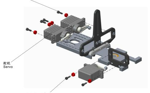
杯头内六角螺丝 Hexagon socket head cap screws M2X6
