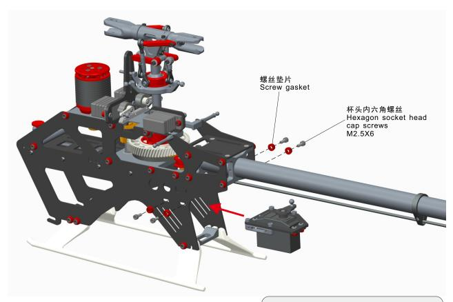
舵机装入机架前需调舵机中位设置好 Please adjust the middle position of the servo's before installing it
